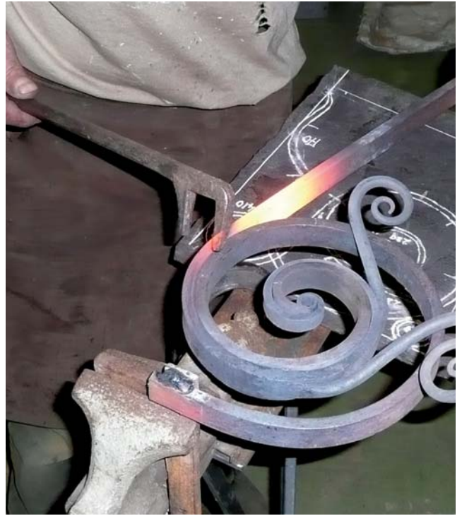
Dorothea craftsmen working the wrought iron balustrades.
